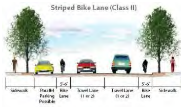
Class II Bike lane section Source: Fehr & Peers, 2010
