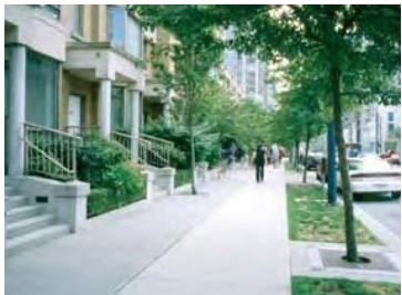
Sidewalk widths should be generous enough to accommodate a curb zone with trees, a circulation zone, and a ground floor related zone that can be used for seating, displays or bike parking.
