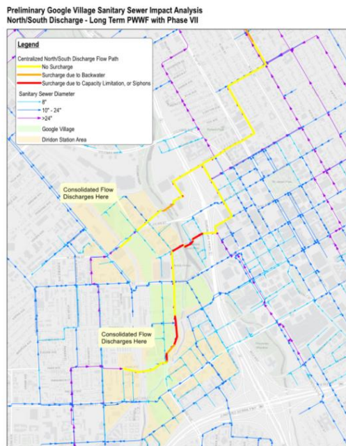
Figure 7.5. Scenario 3, Two WRFs with two points of connection at Park Avenue and West Julian Street
