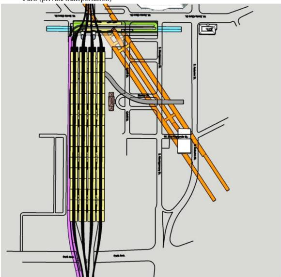
Construction phasing will start with the relocation of the light rail tracks to a tunnel (purple) between Sunol and White Street to the light rail (yellow) platforms located between the concourse and the BART (green) platforms (this configuration is similar to
