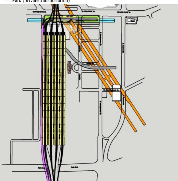
Construction phasing will start with the relocation of the light rail tracks to a tunnel (purple) between Sunol and White Street to the light rail (yellow) platforms located between the concourse and the BART (green) platforms (this configuration is similar to the MUNI Embarcadero station).
