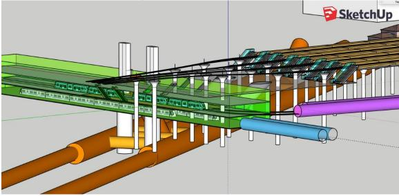
Next, the two west-most heavy rail tracks and platforms will be raised above the area currently occupied by the light rail station and tracks.
